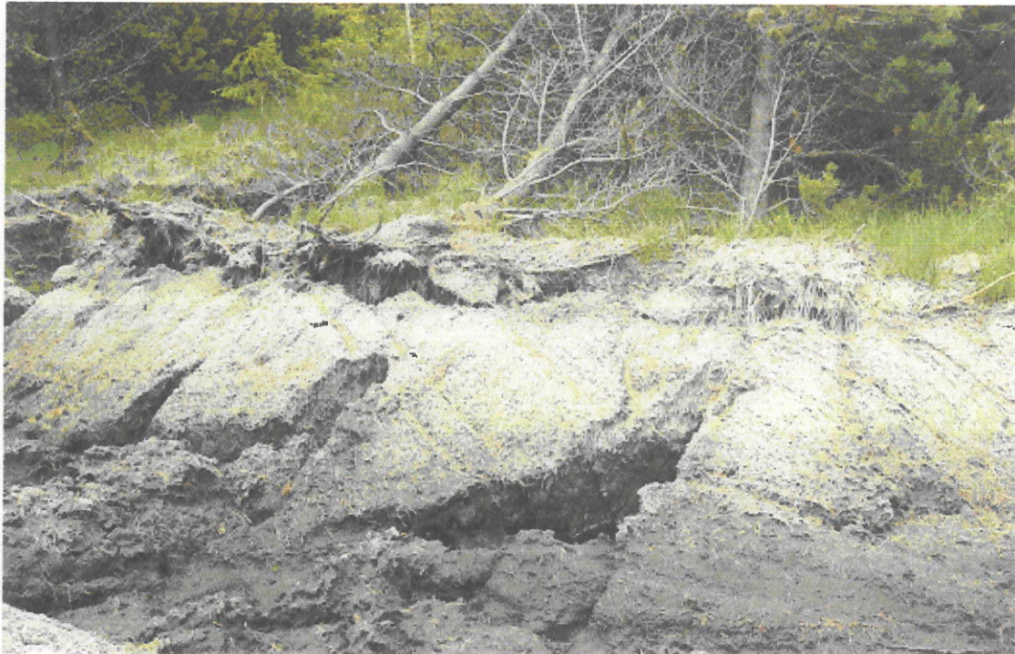
Plate 8.6: Face of delaminated ribbon of peat. Note the depth of delamination and the tendency of tree roots to run along the line of the ribbon with few roots extending laterally at right angles to the ribbon. This suggests that there is relatively limited root growth across lines of the cracks that form under plantation conditions.
