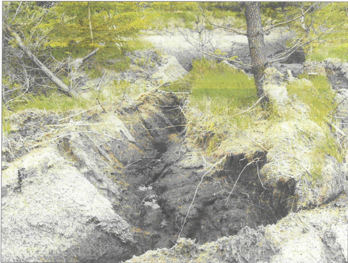
Plate 8.7: Delaminated ribbons of peat at the edge of the failed area near T70. The two-layered structure of the peat profile is obvious on the faces of the ribbons but there are few protruding tree roots. Some cracking of catotelm peat is evident in the upper picture.
