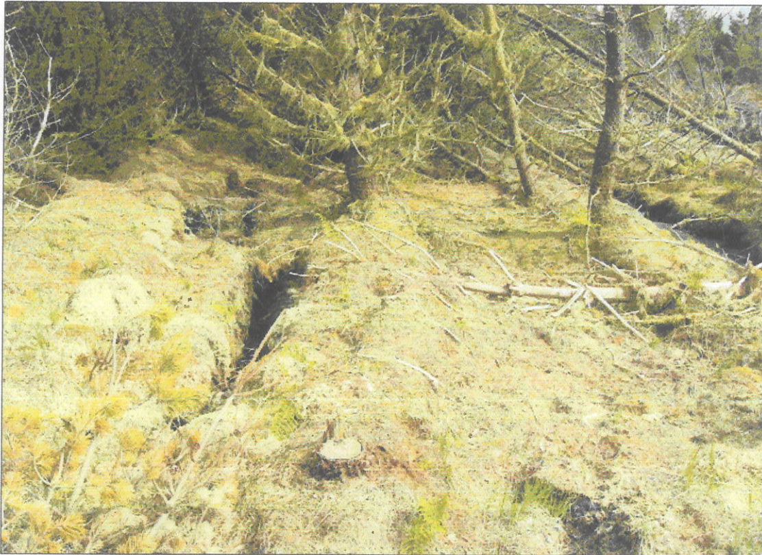
Plate 8.8: A peat ribbon just beginning to separate along what appears to be a plough-furrow crack adjacent to the failed area.
